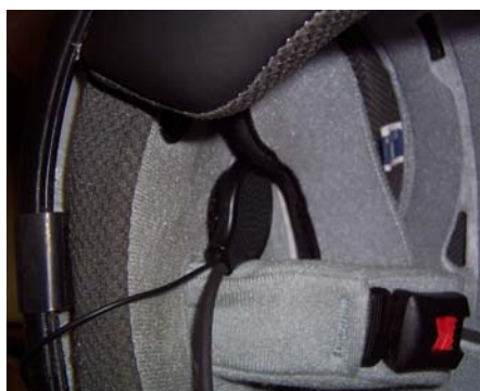
the speaker with short wire cord for left ear
