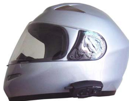
BIM mounted on a helmet
